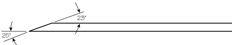
**Figure 5: Blade edge geometry, as supplied.**
