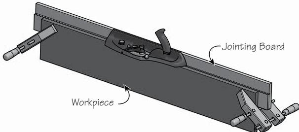
**Figure 7: Jointing board.**
